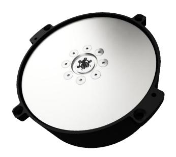
The system relies on a deployable drag sail: by increasing the satellite's aerodynamic surface, atmospheric drag is enhanced, accelerating orbital decay and ensuring a safe and complete destruction of the spacecraft upon re-entry.
